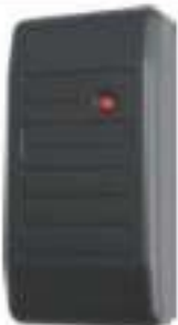
Model: VAL-RF90S-HID Reading Range: 5-375px Communication Distance: WG<100M, RS485<1200M Dimension: 80*48*12.5(mm) Weight: 0.12kg
