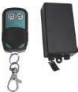
Model: VAL-R16 Contact Output: NONCCOM Transmitting Freq: 433.92MHZ Remote distance: 15m Suitable for: access control Transmitting Distance: ≥70m (in open area) Dimensions: 66Lx45Wx30H(mm) Weight: 0.2kg
